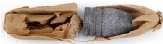
Fig. 12. Confederate .58-cal cartridge, date unknown. Note the internal powder cylinder and the pasted end of the powder case.
